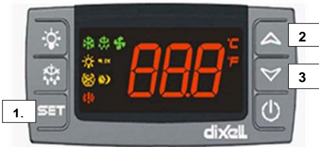
Abb. 3.1: Controller type DIXELL- operating elements and display indicators (symbols)
